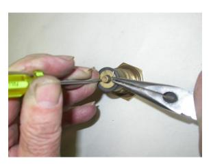
3. Disassemble the fuel valve.
