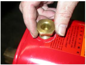
12. Using the ratchet and the holding tool, firmly tighten to recommended torque value (320-350 inch-lbs).
