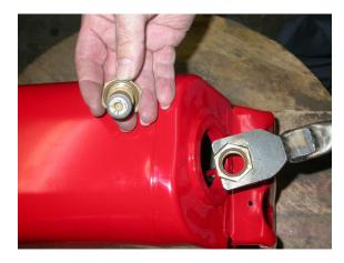
11. Holding the nut with the holding tool, screw in the female valve body.
