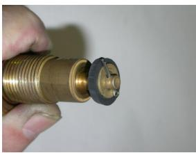
9. Using the pliers and screwdriver, secure the cotter pin on the valve.
